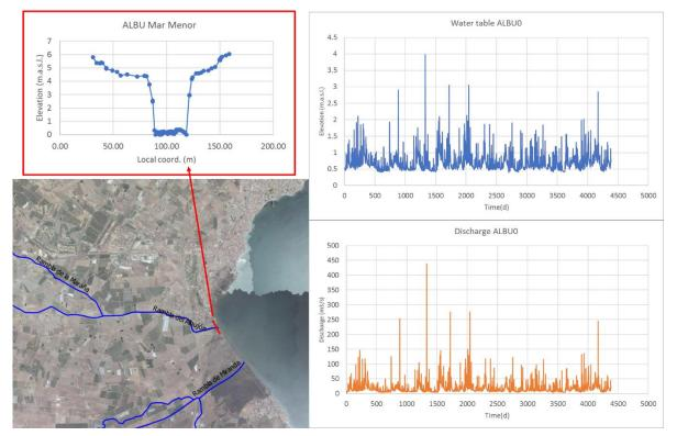
**Summary:** Flood routing is a procedure to determine the time and magnitude of flow (i.e., the flow hydrograph) at a point on a watercourse from known or assumed hydrographs at one or more points upstream. The software BASEMENT (ETHZ) has been used to model a hypothetic flood at the Rambla del Albujón, in Spain. Scenario analysis was carried out, including the implementation of mitigation measures (e.g., river widening) and different inlet hydrographs.
